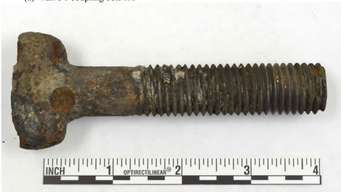
(b) Valve 1 coupling bolt 1B after cleaning
