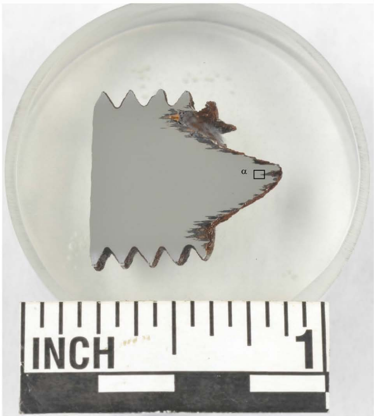
Figure 13 Photograph of the longitudinal section through the end of the valve 1 bonnet bolt prepared for metallography.
