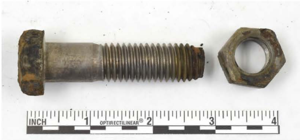
(a) Valve 2 bonnet bolt 2 after cleaning
