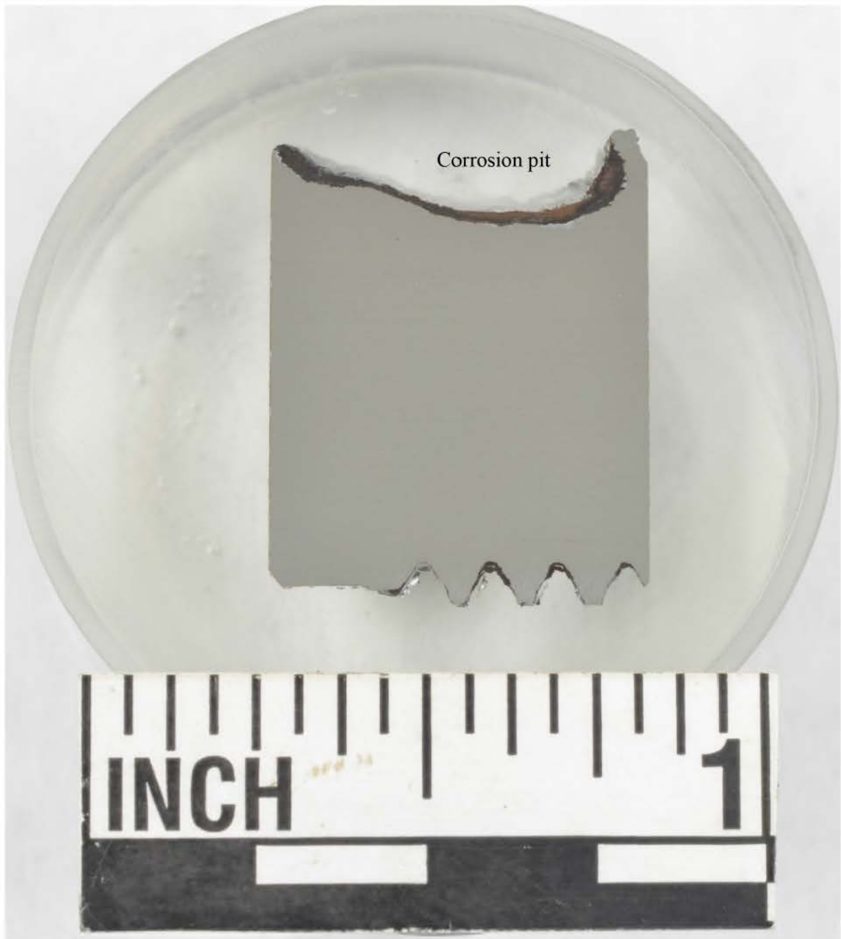
Figure 18 Photograph of the longitudinal section of valve 1 coupling bolt 6A prepared for metallography.
