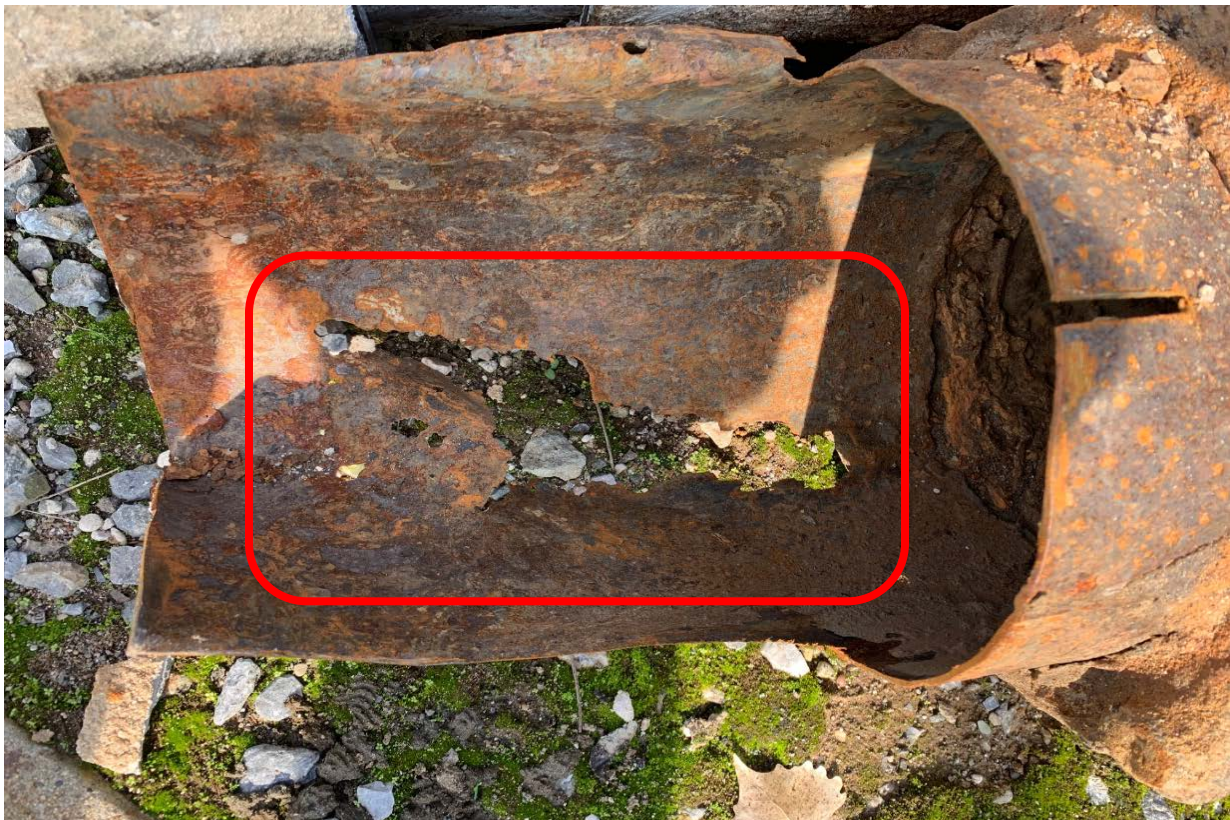
Hole in bottom of 8" MLS pipe
