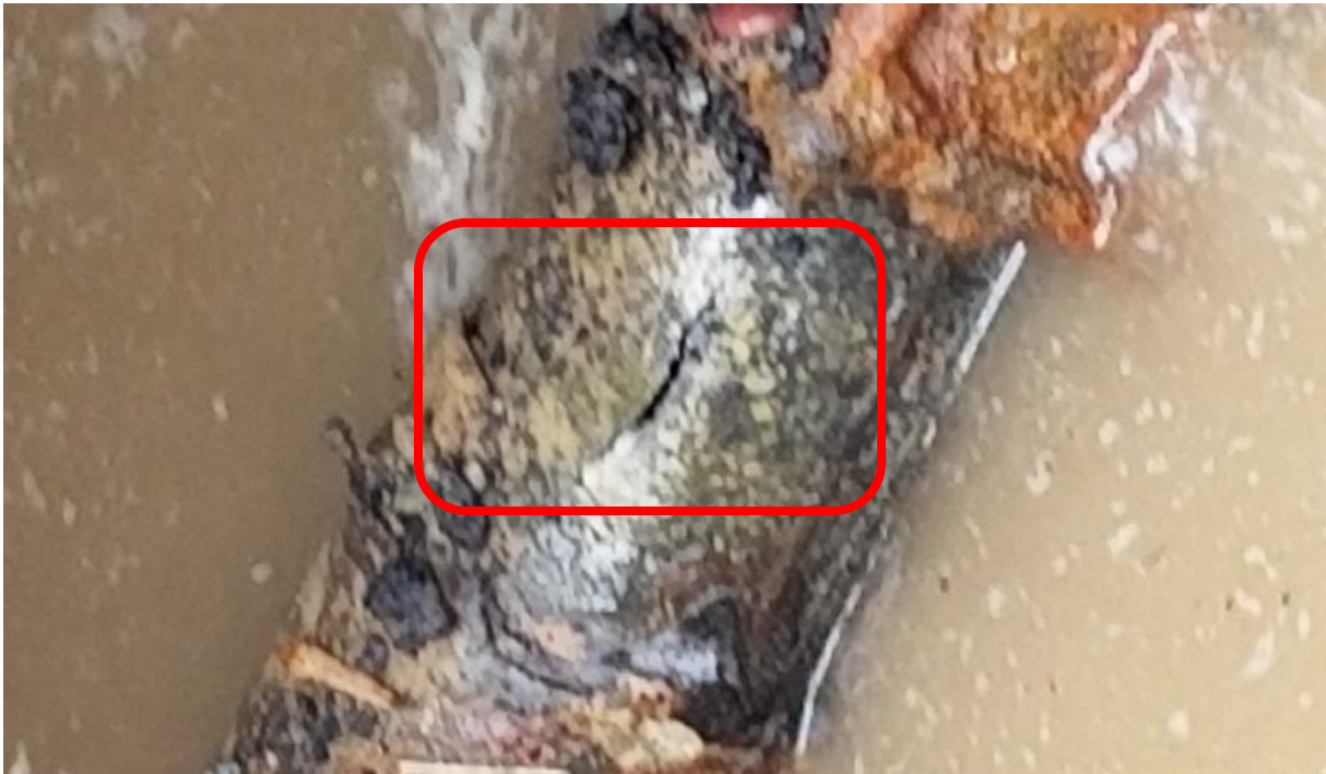
Hole in bottom of 8" MLS pipe
