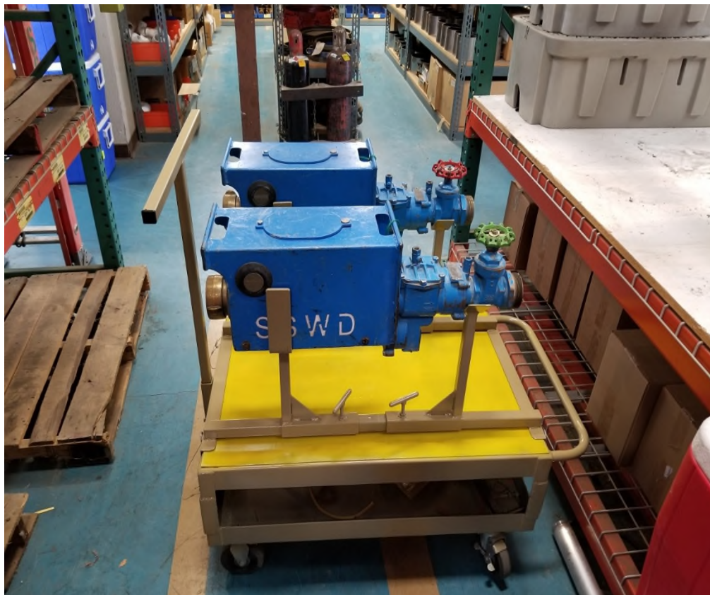
Hydrant Meter Cart with Two Assemblies
